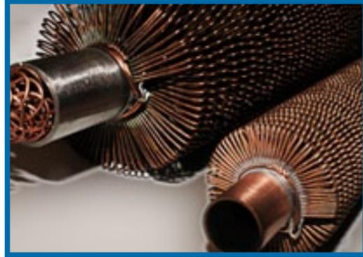
This is our star product and gives a very compact air cooled heat exchanger. Here the Fins consist of Wire loops that are both fastened and soldered to the tube. A specially flattened wire that runs through the base of the wire loop fins does this fastening.
